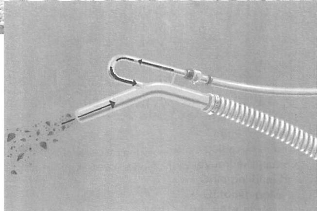
Figure 2. Nozzle of the suction dredge.
